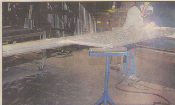
Above, a worker at Aluminum Athletic Equipment in Royersford welds a section of a baseball outfield foul line post.
